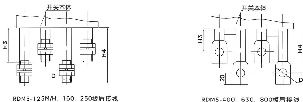
RDM5-125~800板后接线外形及安装板开孔尺寸
